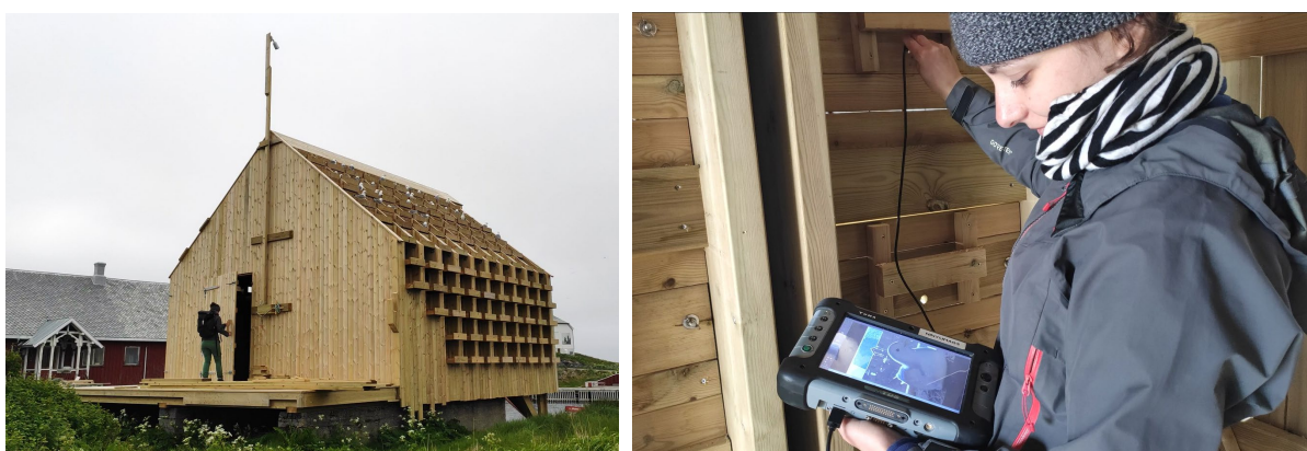
Figure S10. Inspecting nest contents from inside the Kittiwake hotel through a small hole in the back wall of each nest platform, using a USB endoscope connected to a field computer (© Lisa Alcaraz).
