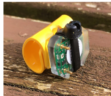
Figure 1. Geolocator attachment rings (yellow) attached to an MK3006 GLS via a cable tie. Self-amalgamating tape is present in between the cable tie and the GLS that is either untrimmed a), or trimmed and ready for deployment, b). White arrows indicate untrimmed self-amalgamating tape in a).
